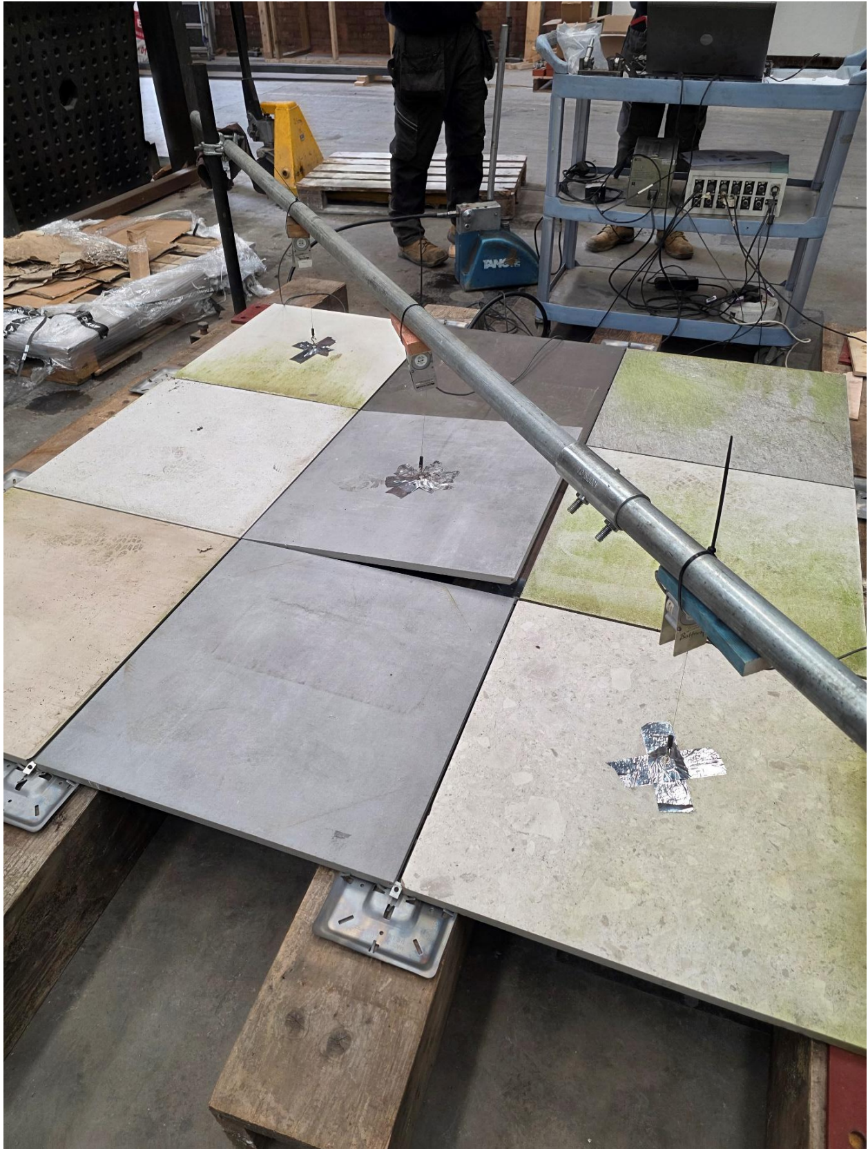
Plate 1 – Test Set-Up and Failure Mode
