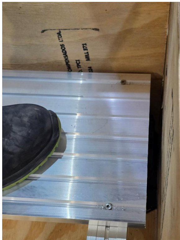
Plate 4 – Base Boards Screwed to Each Rail
