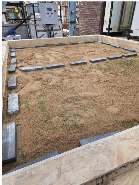
Plate 11 – Weights Added to Hold the Sample Down Whilst the Adhesive Cures
