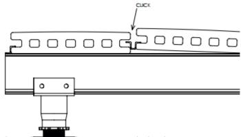
11. Fasten the clips down using the screws provided. The TerraSmart Vitrified Composite Decking is now complete
