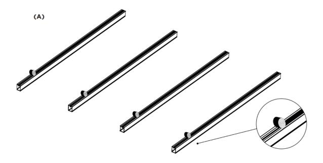
**3.** Lift the joists onto the supports, which should be placed at each end of the joist, and level up to the required height (FFL minus board depth). **Fig B.**
