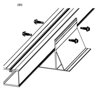
**4.** Add the intermediate supports at the required centres along the joist (as per the joist span, see datasheet). **Fig E.**
