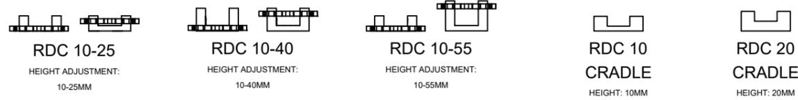
**RDA-C SELF-LEVELLING ADJUSTABLE DECKING PEDESTALS 1:10**
