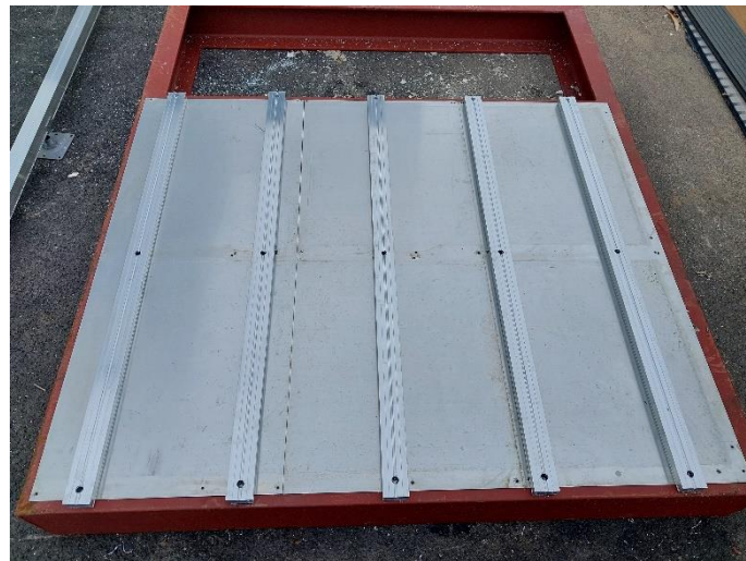
DS Joist Balcony Test Frame with DS25 Joists @ 300mm Centres (Vitrified Composite not shown)
