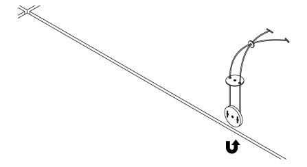
**3.** Insert the clip through the gap between the tiles.
