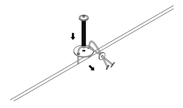
7. Once the clip is fully fastened, pull the tether until it snaps off.
