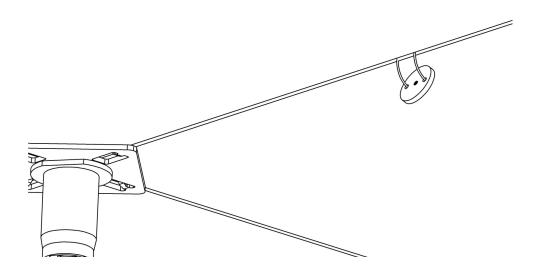
**5.** By lifting the looped tag on the upper section, pull the lower washer tightly against the tile, enabling you to locate and engage the screw.
