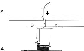
Insert the clip through the gap between the tiles.
