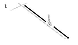
Position the clip at the centre of the gap at each side of the tile.
