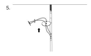
By lifting the looped tag on the upper section, pull the lower washer tightly against the tile, enabling you to locate and engage the screw.
