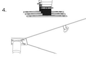
Ensure the bottom washer protrudes beneath the paving completely.
