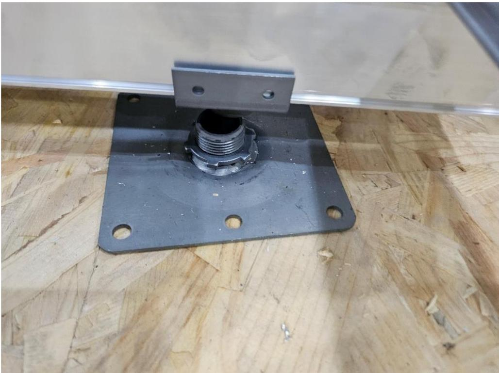
**Plate 26** – A Pedestal that had Worked Loose During Testing
