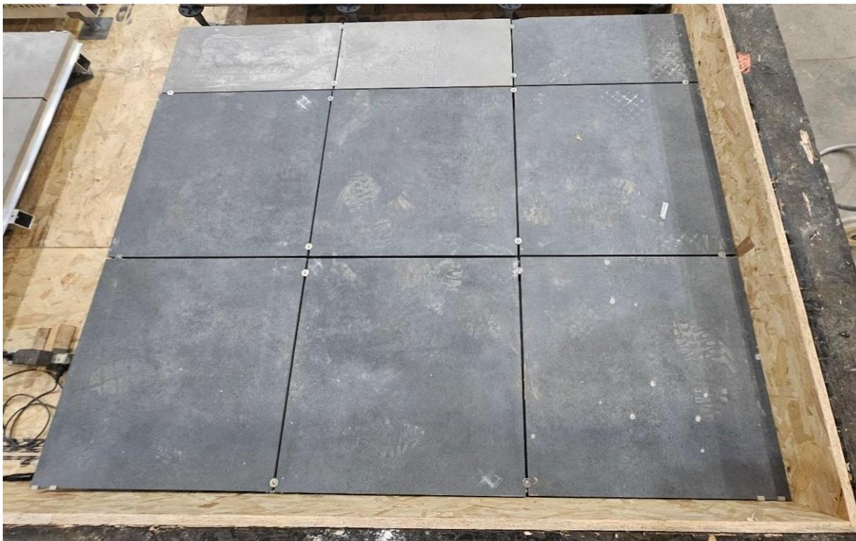
**Plate 22** – Rails and Visual Fix Test Sample Completed
